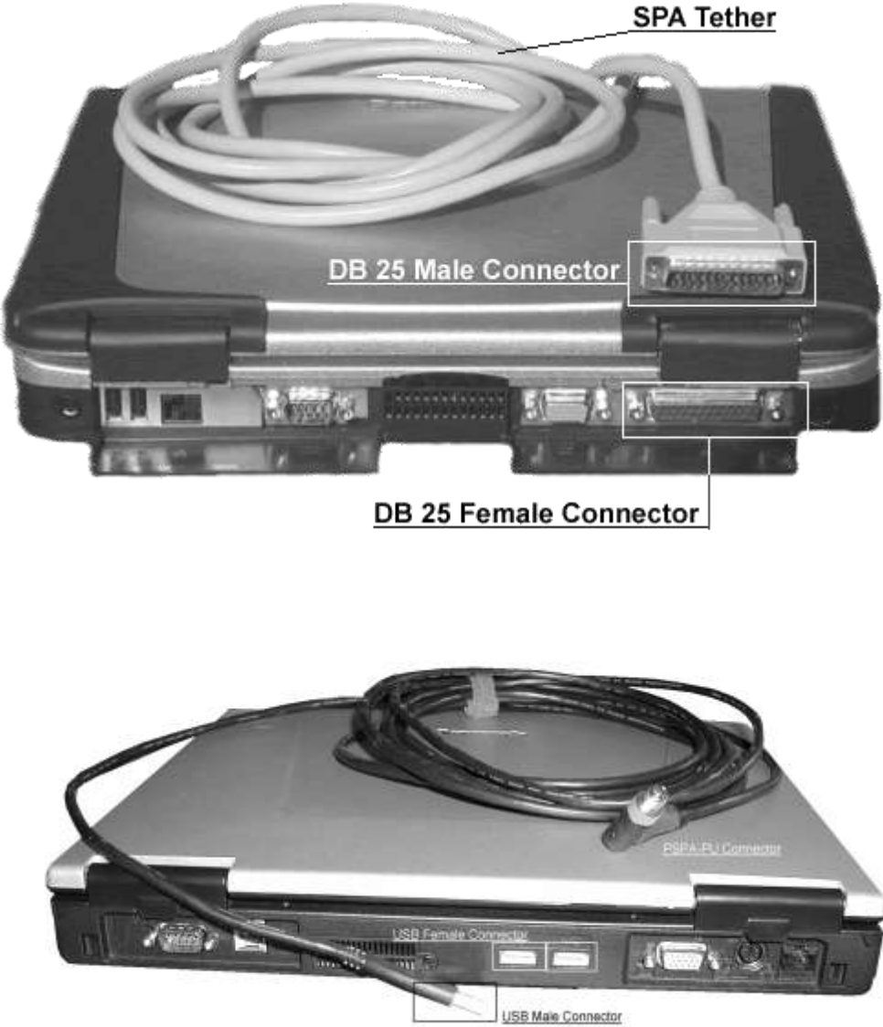
Figure 2.4 The rear of the PSPA-P (a) and PSPA-PU (b) showing the tether connector.
